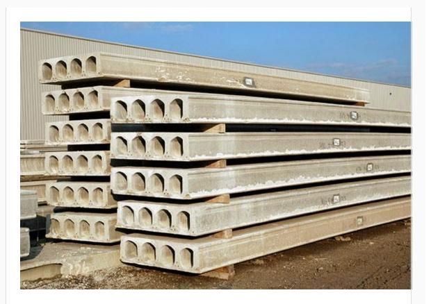
Hollowcore plank is one of the most popular, efficient and versatile components in the construction industry offering architectural and structural design flexibility.
