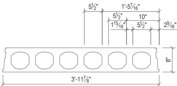
HOLLOW CORE: F<sub>c</sub> = 9000 psi, WEIGHT = 62 psf
